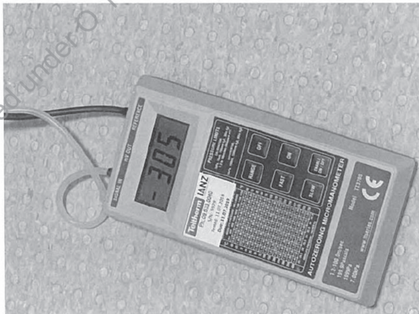
Figure 7: >300 Pa pressure differential reading during testing Unit 3
